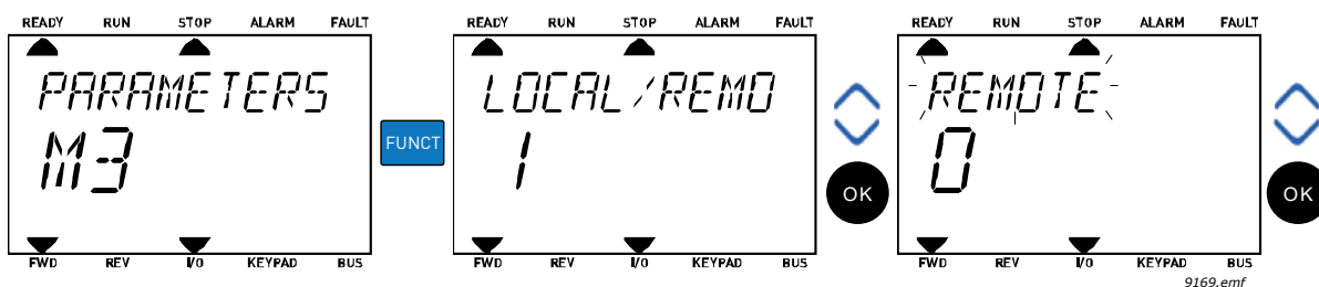
Figure 24. Changing control places
