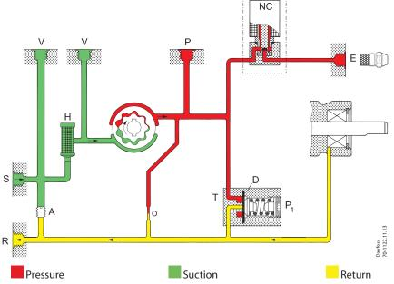
From the suction inlet (S) oil is drawn through the filter (H) to the gear set, where the pressure is increased. When voltage is applied to the NC-valve, it opens and releases oil to the nozzle outlet.
