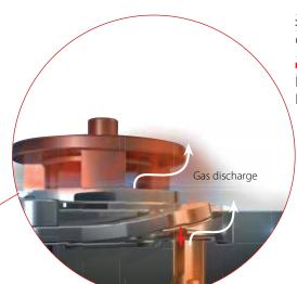
Low Pressure Ratio, part-load, discharge pressure is low, IDVs open
