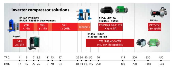
Rating (TR): ARI 45°F / 145°F / SH 20°F / SC 10°F Rating (kW): EN12900 5°C / 50°C / SH 10K / SC 0K - data at max speed for inverter scrolls Rating conditions are for Scroll compressors only.
