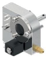
Danfoss COM active oil level regulators use hall effect sensor and built in magnetic float technology for very precise oil level sensing. This design ensures reliable performance even with foaming or dirty oil and long life of the compressor even under different operating conditions such as defrost cycles and seasonal variations.
